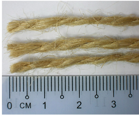
Figure 4. Twisted jute yarn with Tex of 1500. This figure is published in color in the online version.
